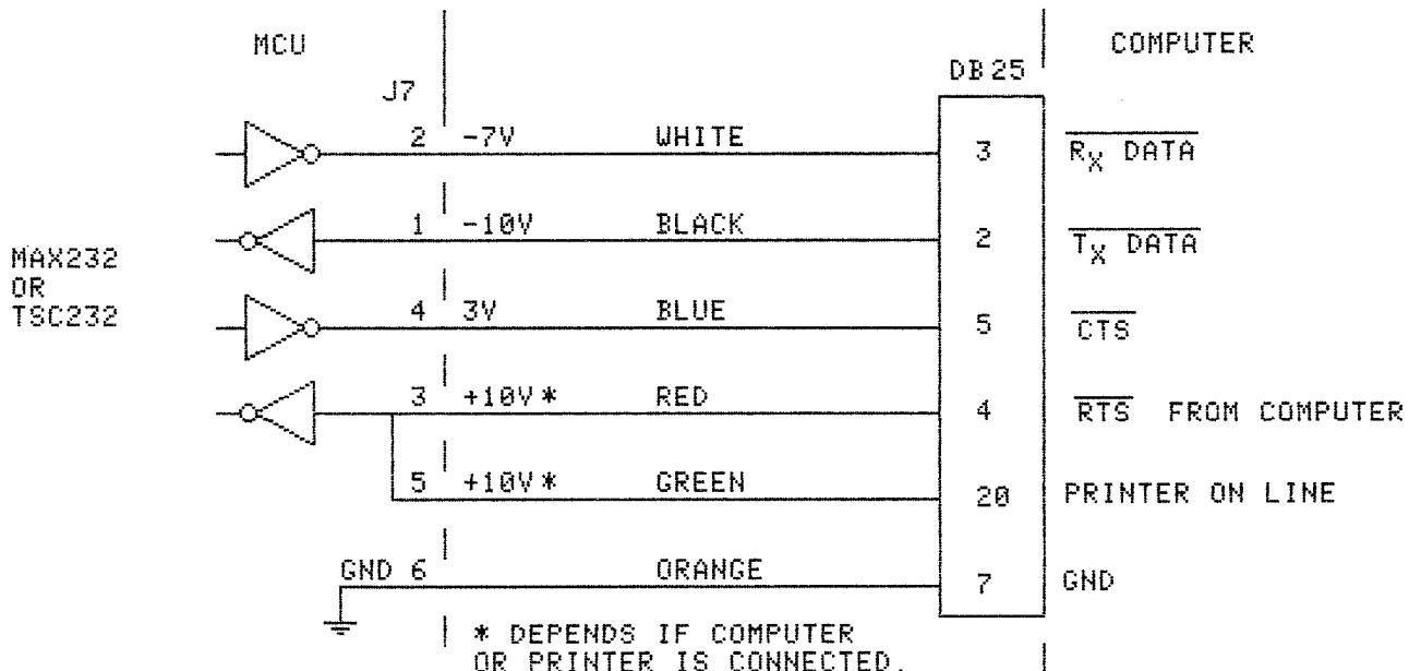
NOTE: THESE VOLTAGES ARE MEASURED IN THE MCU AT J7 (BOTTOM RIGHT CORNER) WITH THE SERIAL CABLE CONNECTED TO THE FACILITY COMPUTER.
